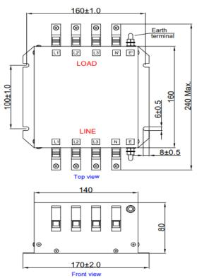
All dimensions in mm General tolerance=±2mm
