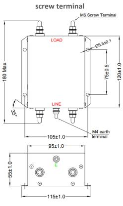
All dimensions in mm General tolerance=±2mm
